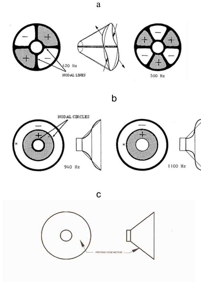
*Fig. 1 - Resonance phenomena in unenclosed loudspeaker cones:*
